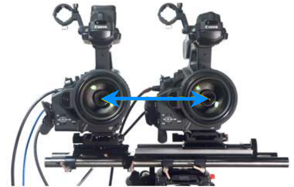
Interaxial Separation between lenses, a.k.a. Stereo Base, a.k.a. Interocular separation, (IPD for human eye)
